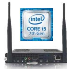
The Open Pluggable System is the Intel standard and allows for a variety of options with regards to chipset, memory, and storage.
