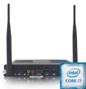
The **Intel® Open Pluggable Specification (OPS) PC with G3 Intel® Core™ i7 Processor** features a 10th Generation "Comet Lake" Intel® Core™ i7-10510U Processor, with 8GB of 2400MHz DDR4 RAM (up to 32GB), an ultra fast 128GB SSD Drive (up to 512GB), crystal clear 4K imagery at 60Hz playback and an HDMI Out, secondary display connection.
